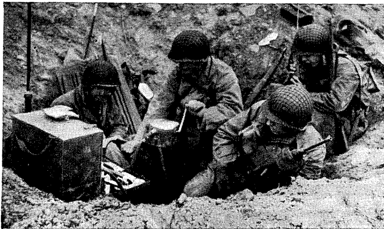
SHELL-HOLE RADIO. A U.S. shore fire control party directing by wireless the fire of Naval guns during the Normandy landings. Note the hand-driven generator. The operator on the right is using a "handie-talkie."
